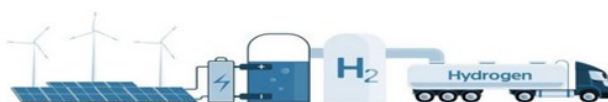
Figure 2 – Supply chain of green hydrogen production from water electrolysis by renewable electricity (Ref.:Azocleantech.com, 2022)
