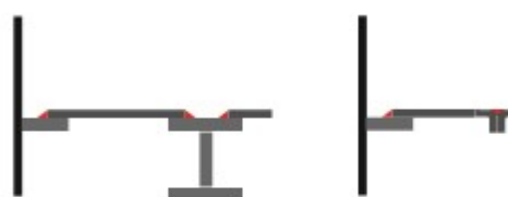
Fig. 10: Construction without thermal compensation
