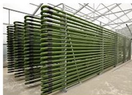
Photo 2-Photo bioreactor (closed-loop) from glass tubes.
