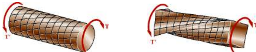
Figure 39 : comparison of deformations in circular and square shafts
