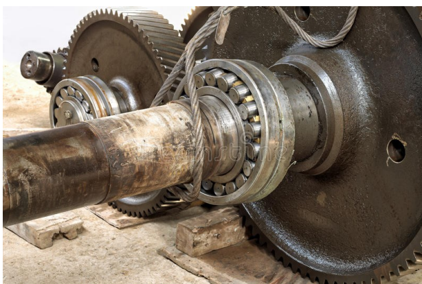
Figure 1. Bearings dislodged from containment
