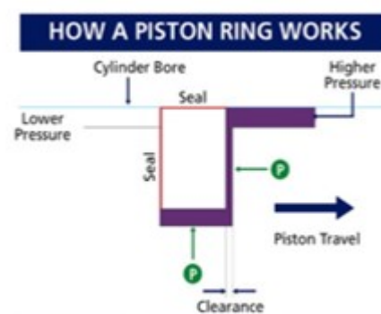
Figure 2. Piston Ring Working
