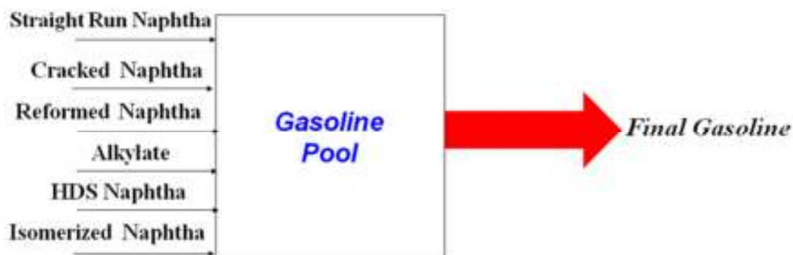
Figure 1 – Example of Process Streams Blending to Produce Gasoline
