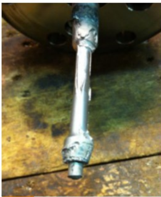
▲ Sulfuric acid corrosion on a stainless steel valve spindle
